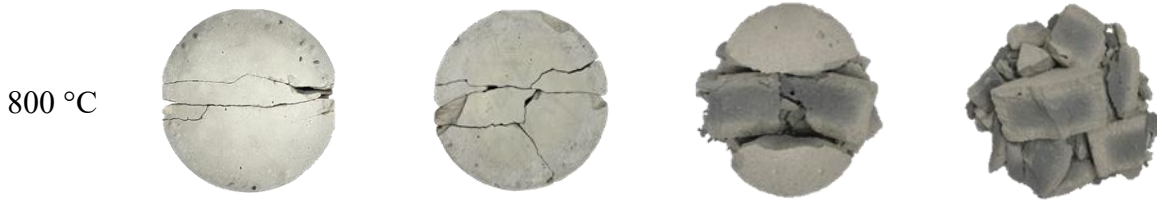
Fig. 10. Failure patterns of ECC specimens under various strain rates.
