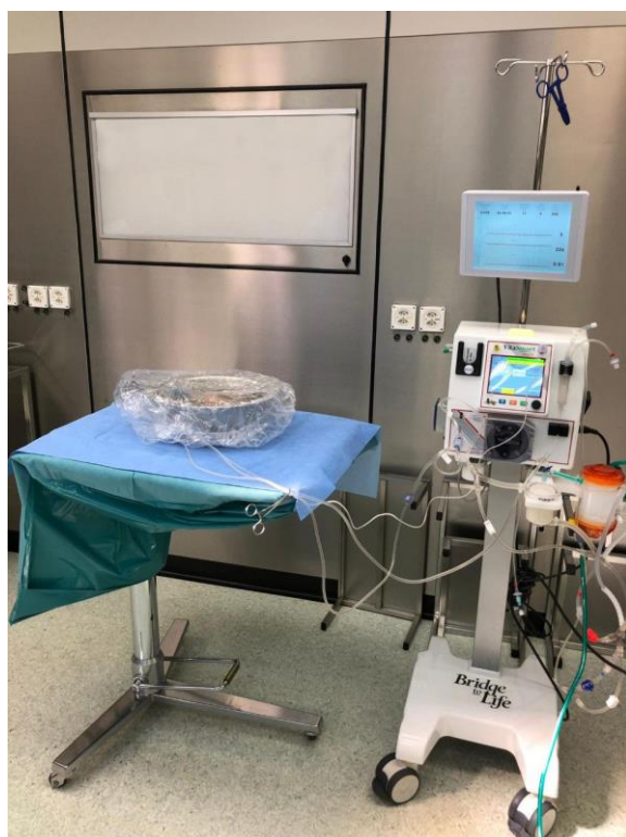
Figure 2. An example of liver HMP for clinical DHOPE (Vitasmart). The main console houses the pump, filter, oxygenator and control panel, with a display panel for continuous readout. The liver is housed in the ice-cooled bowl covered by the sterile drape. (Image provided by Bridge to Life).
