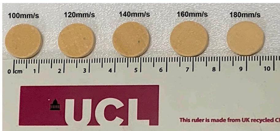
Fig. 1. Images of cylindrical printlets from speeds 100–180 mm/s (left to right).
