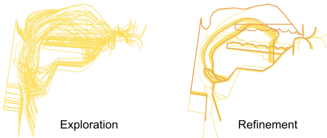
Figure 19 Illustration of the two-step optimisation process. Step 1 Exploration: Uniform random parameter search; Step 2 Refinement: Random parameters search around good solutions.
