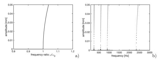
Figure 4. a)Nonlinear free vibrations. b) Nonlinear forced vibrations. By neglecting the nonlinear mass terms  $m_3$ , e.g. valid only for large plates. Radius R increases from right to left.
