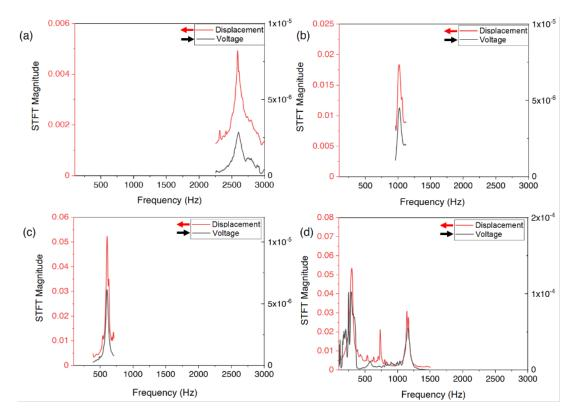
Figure 7. Short-time Fourier transforms for plates with R of a) R = 5 mm, b) R = 8 mm, c) R = 10 mm, d) R = 15 mm. Continuous lines refer to the right axis and the dashed ones to the left axis.
