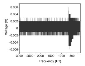
Figure 8. Voltage-frequency signal of an unpoled PVDF film of R = 15 mm collected under SPL level of 112 dB on average.
