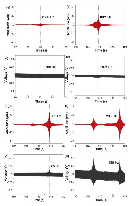
**Figure 6.** Displacement amplitude-time and voltage-time signals during the frequency sweep for the plates with h = 0.110 mm and R of a), c) R = 5 mm; b), d) R = 8 mm; e), g) R = 10 mm; f), h) R = 15 mm.
