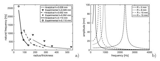
Figure 3. a) Linear natural frequencies as a function of the plate radius R. b) Harmonic response functions for each radius considering h = 0.110 mm.
