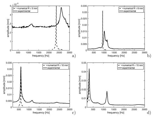
Figure 5. Frequency sweep of the nonlinear system with  $m_3 = 0$  compared to the experimental results: a) R = 5 mm, b) R = 8 mm, c) R = 10 mm, d) R = 15 mm.
