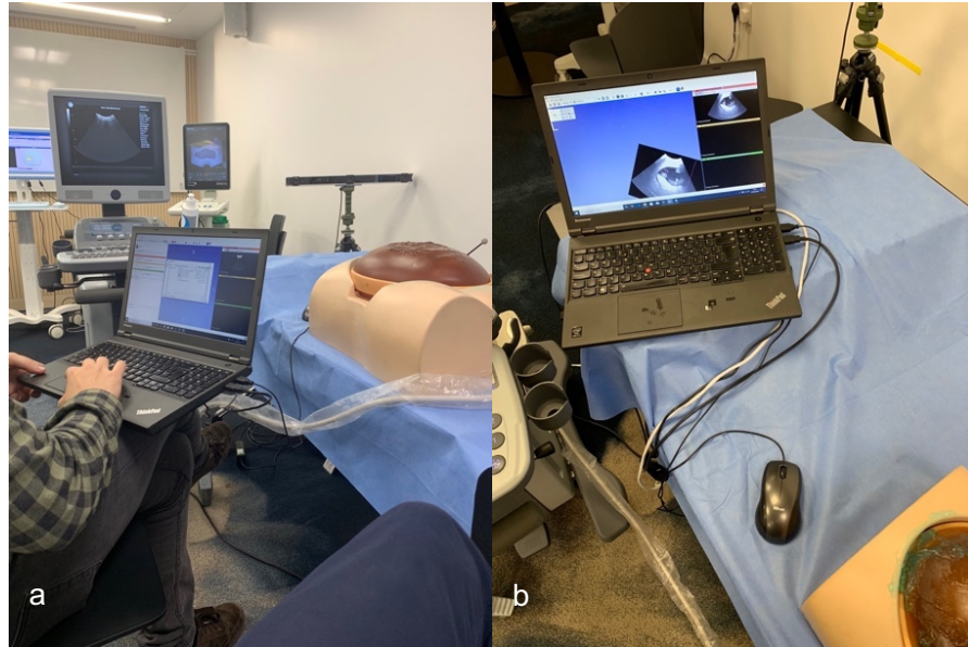
Figure 6.5– Initial mock-up using '3D Slicer', optical tracking and an ultrasonix US system.
