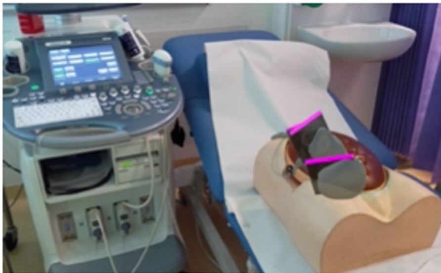
Figure 6.13 - User view of the clinical training environment when they are wearing Hololens with CAL-Tutor software running. To the left is the clinical US system manufactured by GE Voluson and to the right is the training phantom with the fetus overlaid and the standard planes highlighted.
