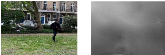
Figure 2: left image: Flying drone with a dynamic obstacle moving toward it (a person running). Right image: Grayscale video reconstructed from events recorded from the same scene
