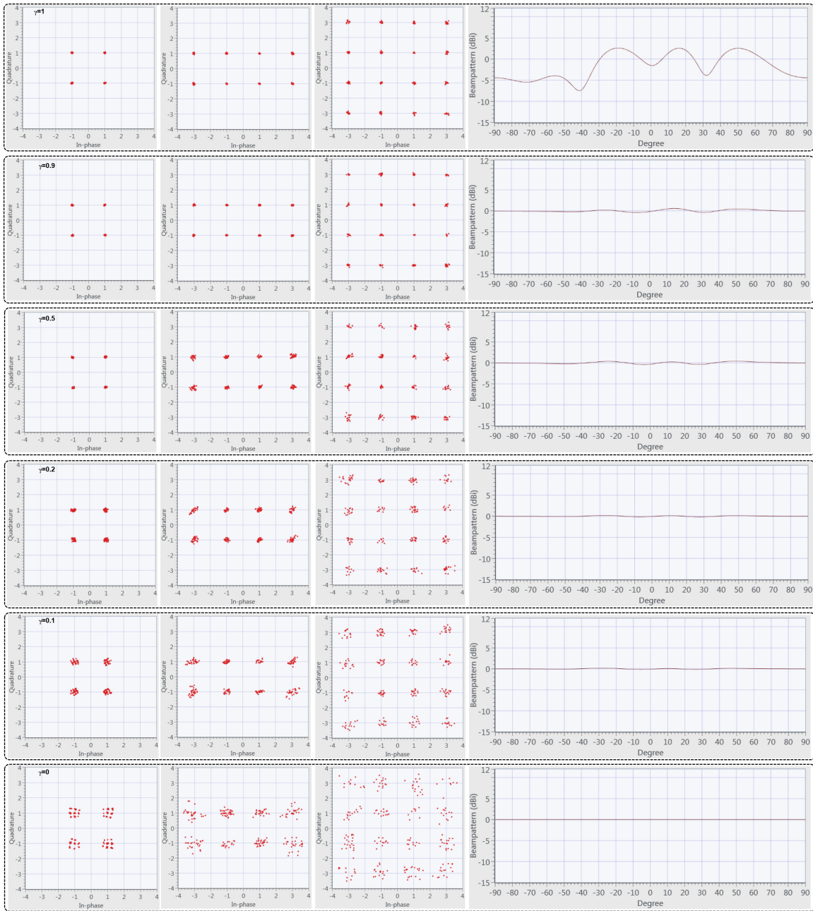
Figure 3: Measurement results at user side in terms of constellation diagram patterns (QPSK, 8QAM, 16QAM) and Tx-USRP side radar omnidirectional beampatterns at different values of trade-off factor \gamma .
