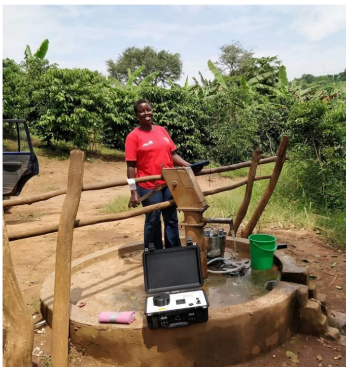
Figure C-4 Low-cost portable fluorimeter used to test the quality of water sampled from a shallow well by co-author Jacintha Nayebare in Lukaya, Uganda; the fluorimeter is contained within the open black hardcase in the foreground of the photo.
