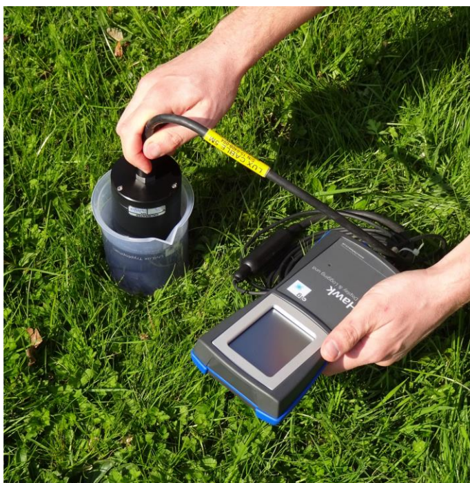
Figure 1-3 UviLux Fluorimeter developed by Chelsea Technologies Group Ltd., UK. Note that the sensor operates using UV light and is sensitive to sunlight; hence, the beaker would need to be covered for a reliable measurement.
