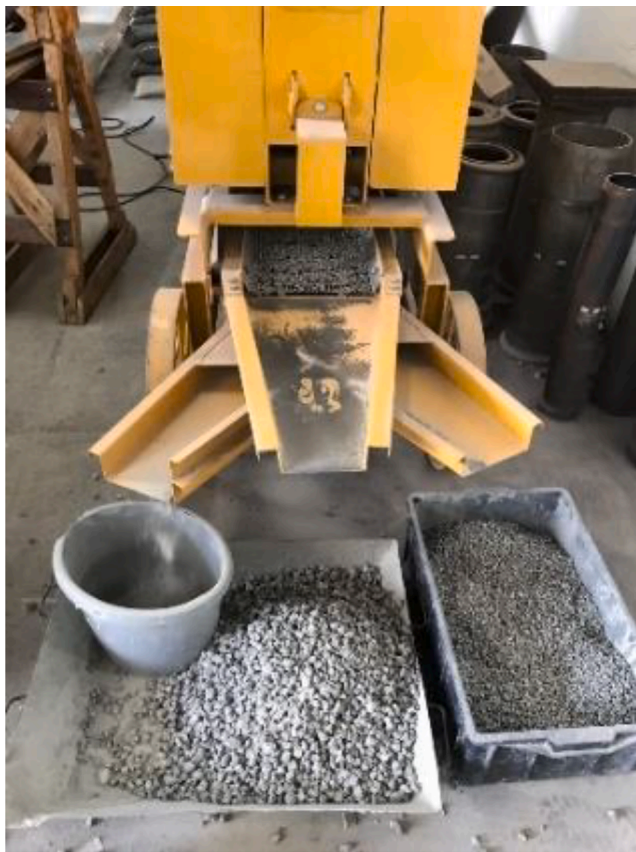
Fig. 3. Crushed concrete used as aggregate in the RAC.
