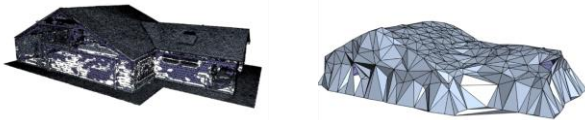
Figure 5: BPA 3D reconstruction of the detached house for the original point cloud (left) and the subsampled one (right).
