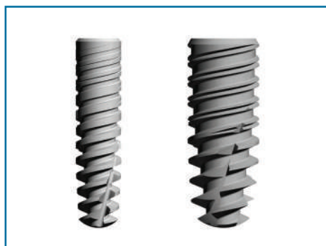
FIG. 1: Drawings showing the difference in diameters of the implants used in the present study: on the left the 3 mm-diameter and on the right the 4 mm-diameter implant.
