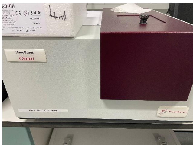
Figure 7.1: Dynamic Light Scattering (DLS) apparatus: Courtesy of UCL School of Chemical Engineering.
