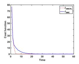
Fig. 7: The cost function J(k) in the simulation test.
