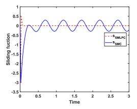
Fig. 17: The sliding function s(k) in the simulation test.
