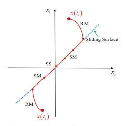
Fig. 1: Phase diagram of continuous SMC.
