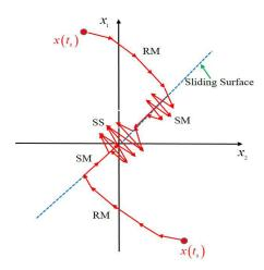
Fig. 2: Phase diagram of a discrete SMC.
