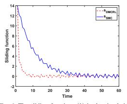
Fig. 6: The sliding function s(k) in the simulation test.
