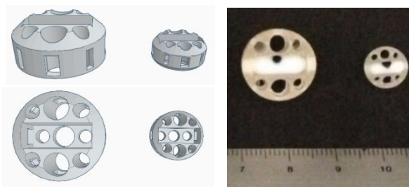
Figure 2. Designed Carousel (Left) and Microwave (Middle) devices and their final 3D Printed congeners (Right).
