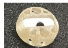
Figure 3. 3D Printed Carousel Stirrer devices containing 0.5% w/w Pd(PPh 3 ) 4 .
