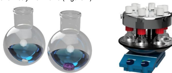
Figure 1. Illustration of the concept of 3D Printed Catalytically active Stirrers, against traditional batch catalysis (Left) and the 3D Printed variant (Middle) and their clear utility when used in carousel format (Right).
