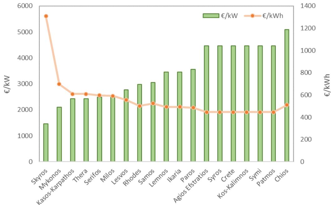
Figure 4.18: Total BESS built costs per kW and kWh for each Electrical System
