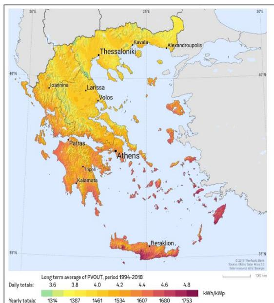
Figure 4.8: Photovoltaic power potential in Greece (The World Bank, 2019b)
