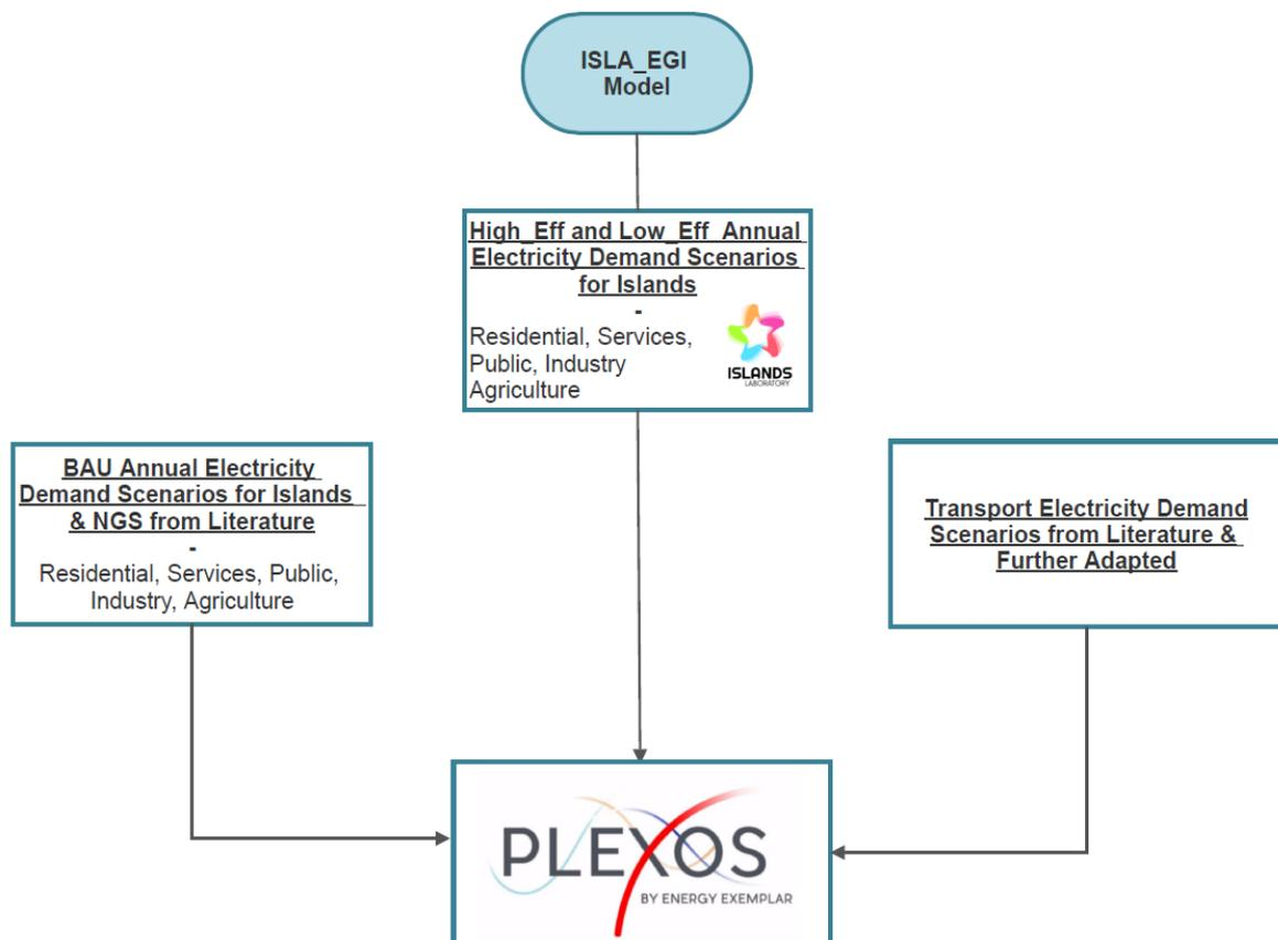
Figure 3.1: ISLA\_EGI soft-linking with PLEXOS energy system model
