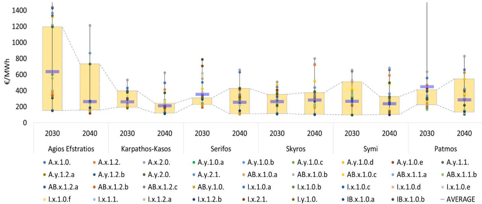
Figure 5.44: Levelized costs of energy produced by small-sized island electrical systems for 2030 & 2040
