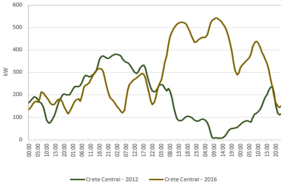
Figure 4.6: Simulated hourly output for the same week in August 2012 and 2016 from 1 MW W/T in Central Crete (Pfenninger, S., Staffell, 2018)
