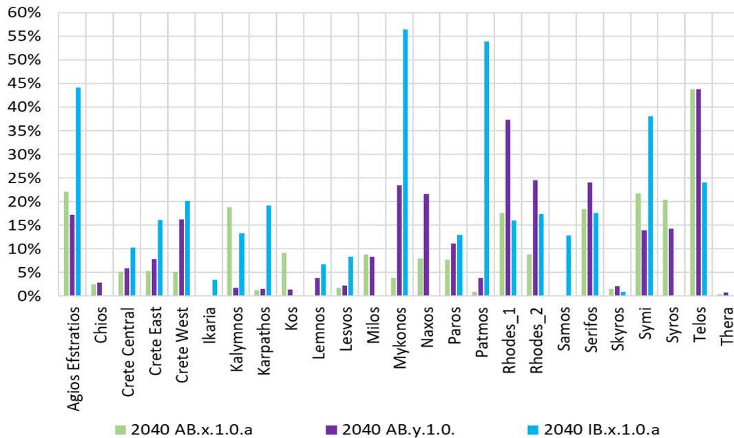
Figure 5.22: Capacity factor for BESS utilisation in 2040
