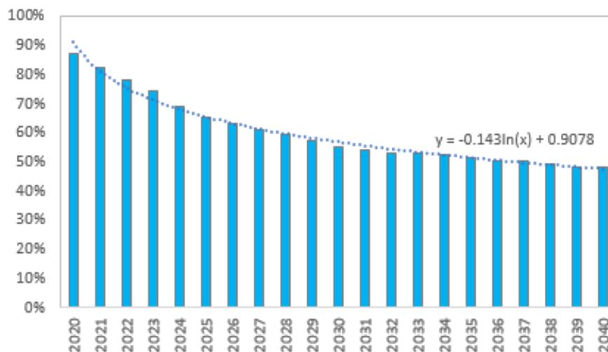
Figure 4.17: Cost reduction for battery cells as a percentage (%) of 2017 reference prices (Cole *et al.*, 2019)
