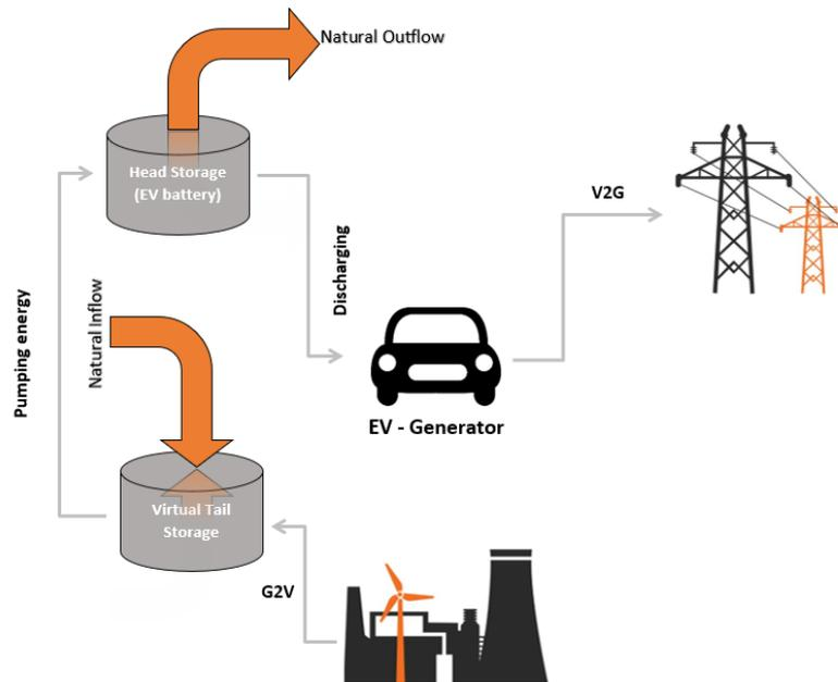
Figure 4.27: V2G schematic applied in PLEXOS model
