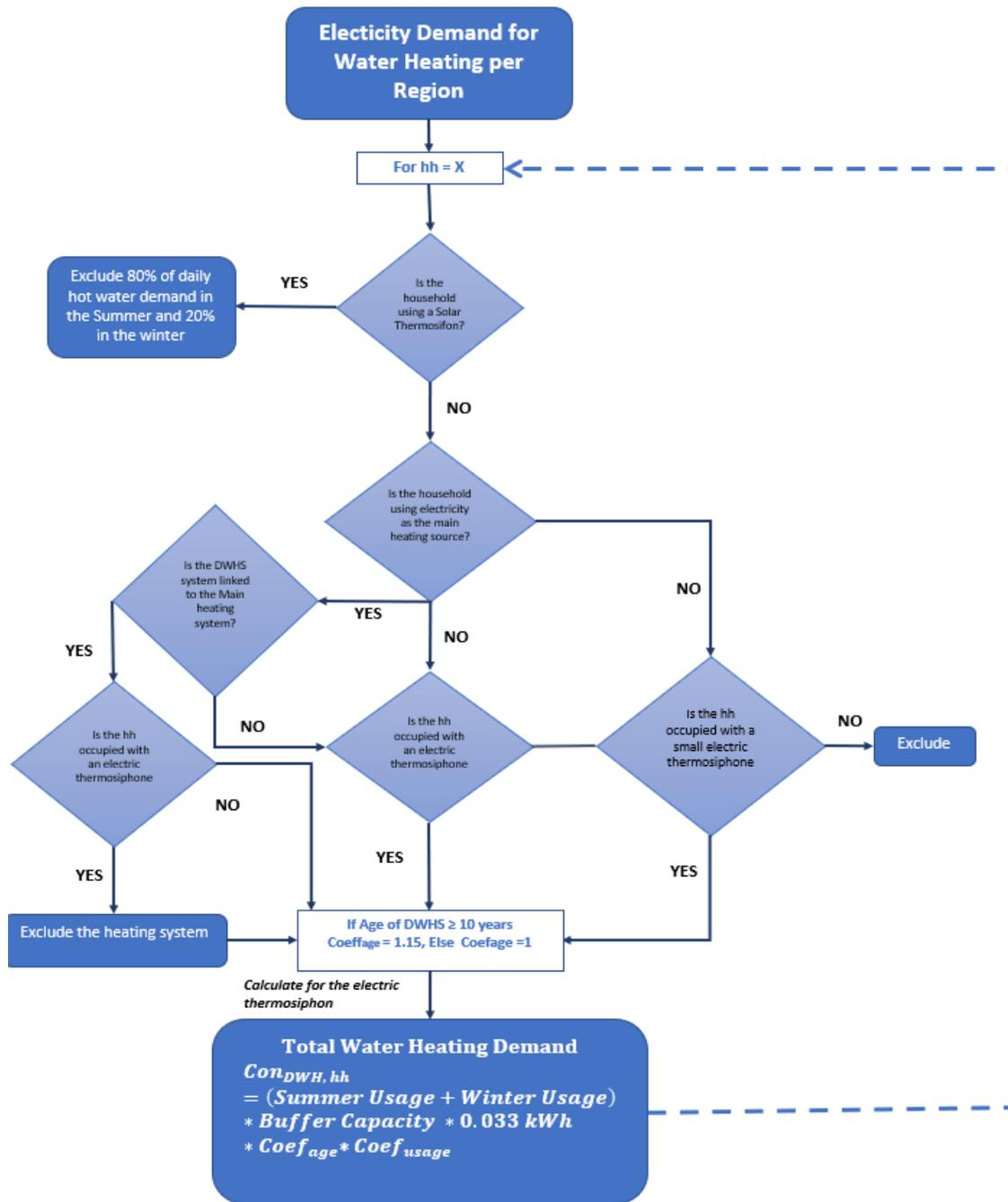
Figure 3.15: Flow chart for calculating water heating electricity demand in the residential sector
