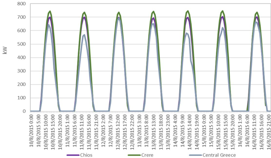
Figure 4.5: Simulated hourly output for one week from 1 MW of PV solar systems (Pfenninger, S., Staffell, 2018)
