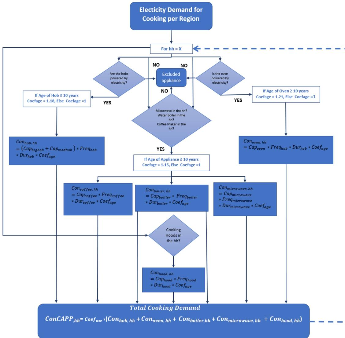
Figure 3.26: Flow chart for calculating electricity demand for cooking in the residential sector
