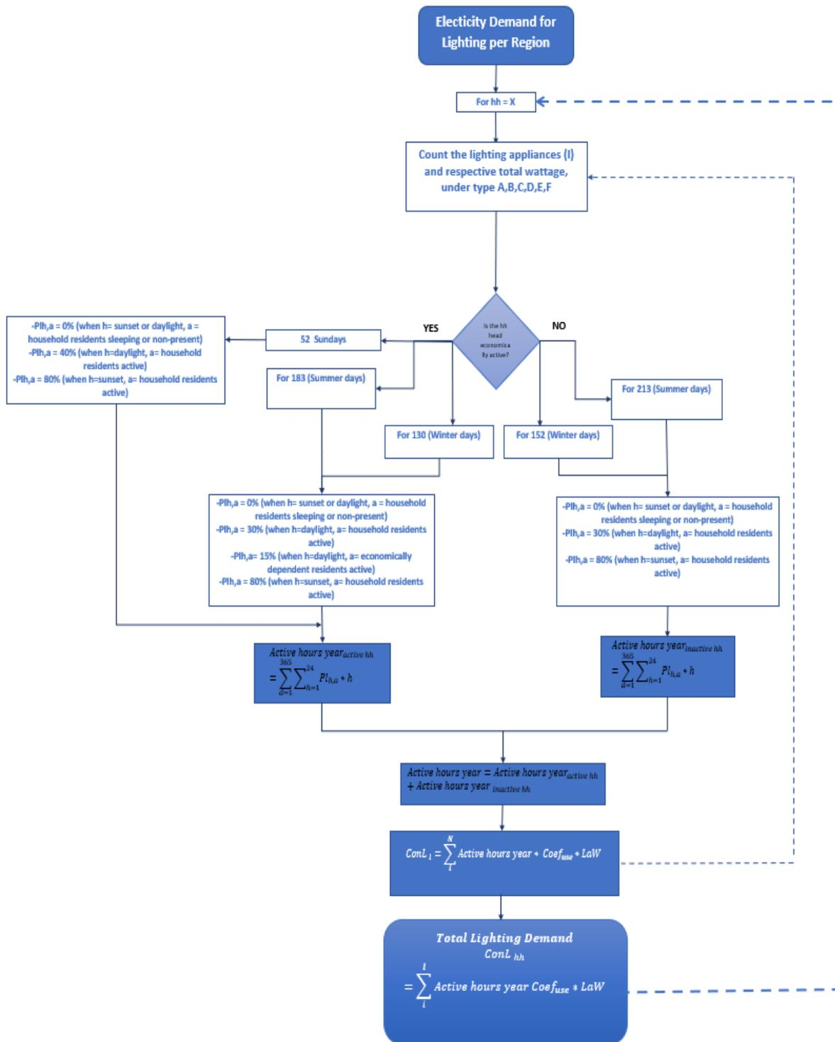
Figure 3.17: Flow Chart for calculating lighting electricity demand in the residential sector
