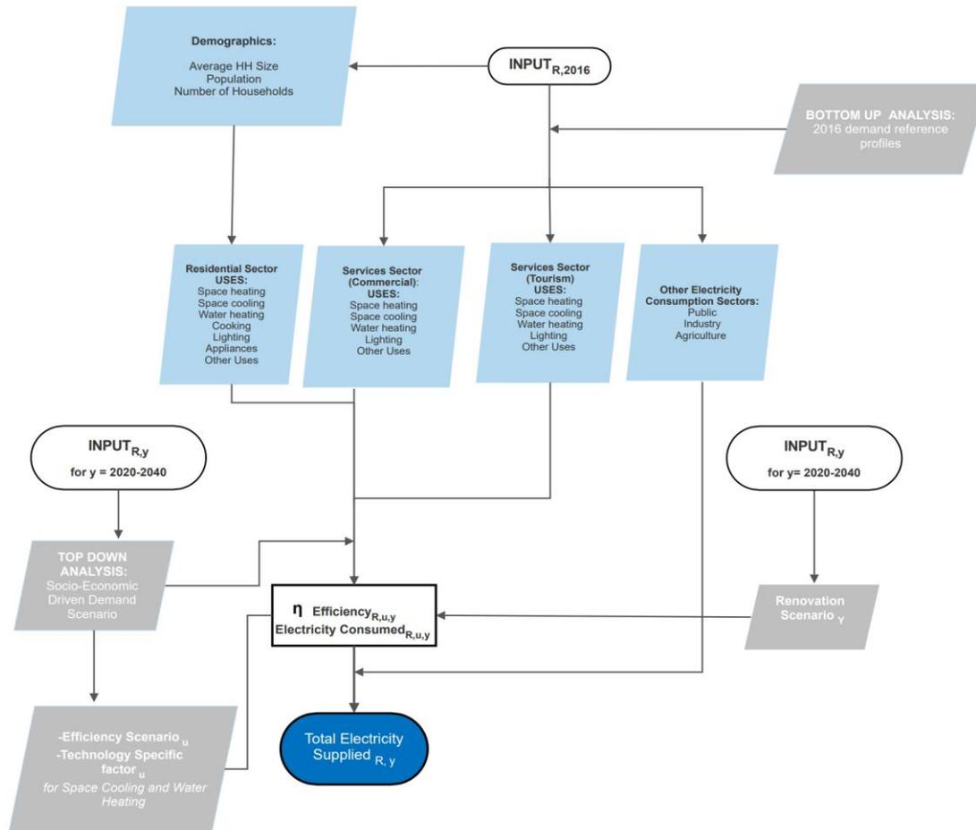
Figure 3.3: Flow chart of data processing and ISLA\_EGI model adapted for the Greek islands
