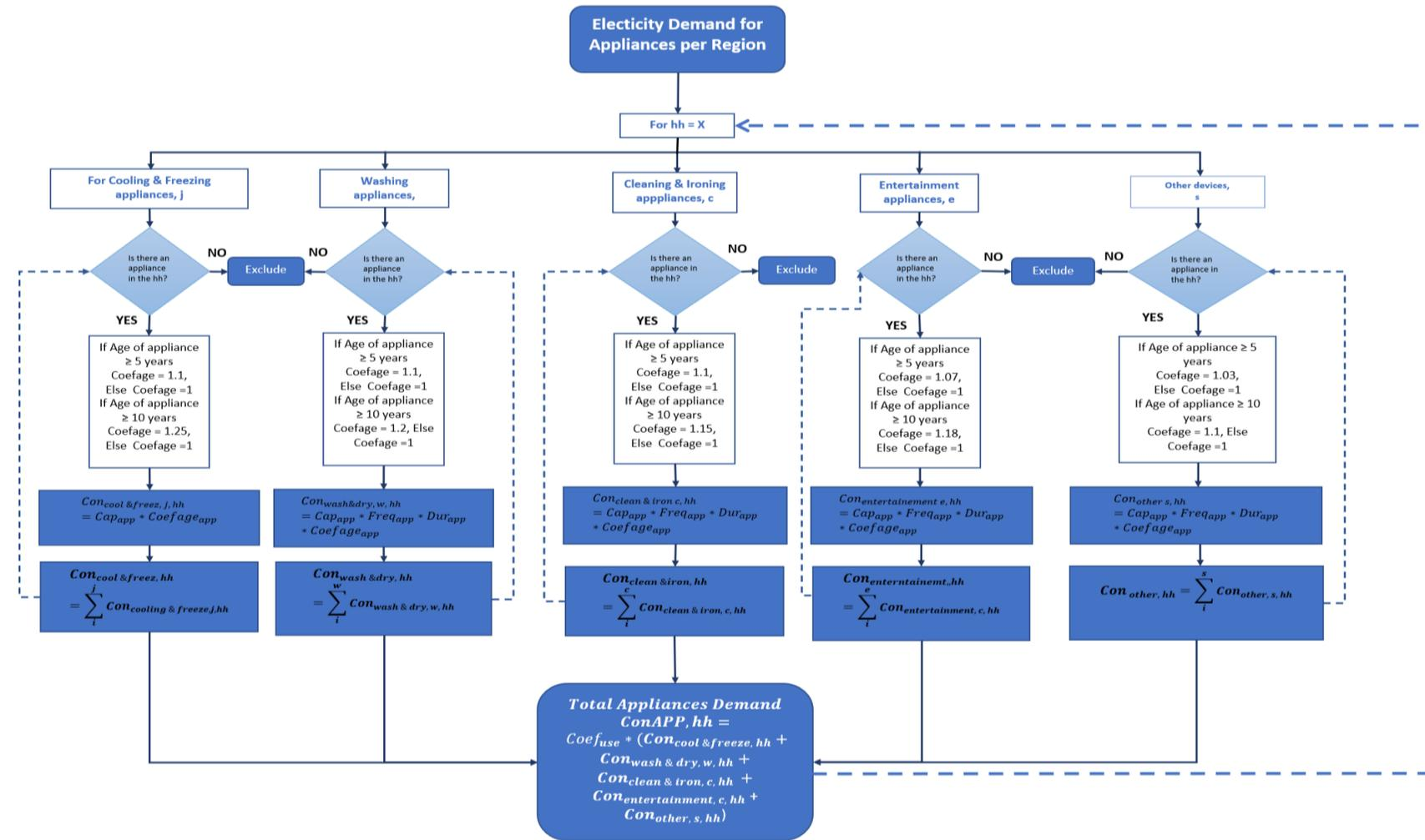
Figure 3.24: Flow chart for calculating appliances electricity demand in the residential sector
