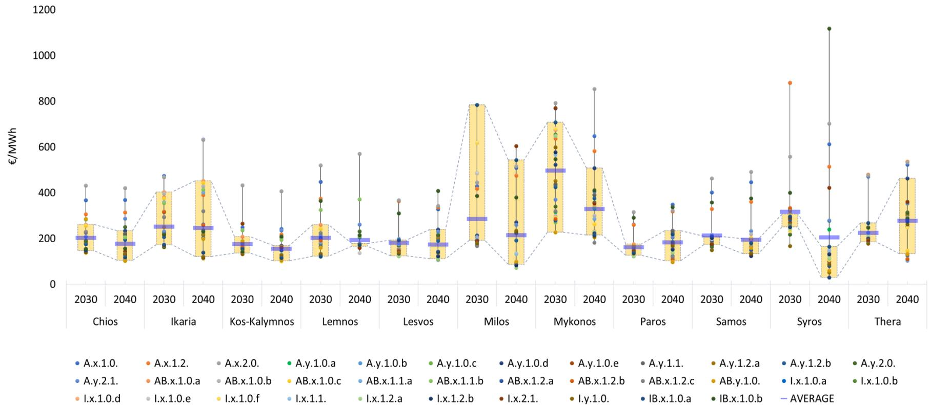
Figure 5.43: Levelized costs of energy produced by medium-sized island electrical systems for 2030 & 2040
