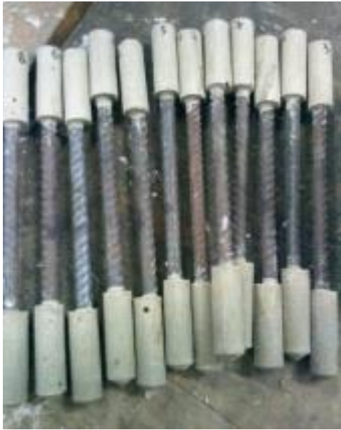
(e) Steel bars with mortar end caps
