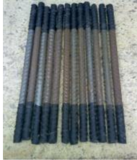
(b) Steel bars wrapped in self-amalgamating tape at both ends
