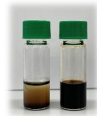
Figure 1. Photograph of \text{Cu}_3\text{N} nanocrystals after regular (left) and optimized (right) purification.
