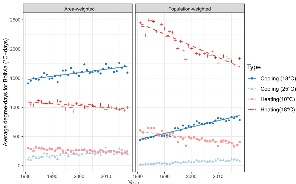
Fig. 6. Area-weighted and population-weighted degree-days for Bolivia by year at given base temperatures.
