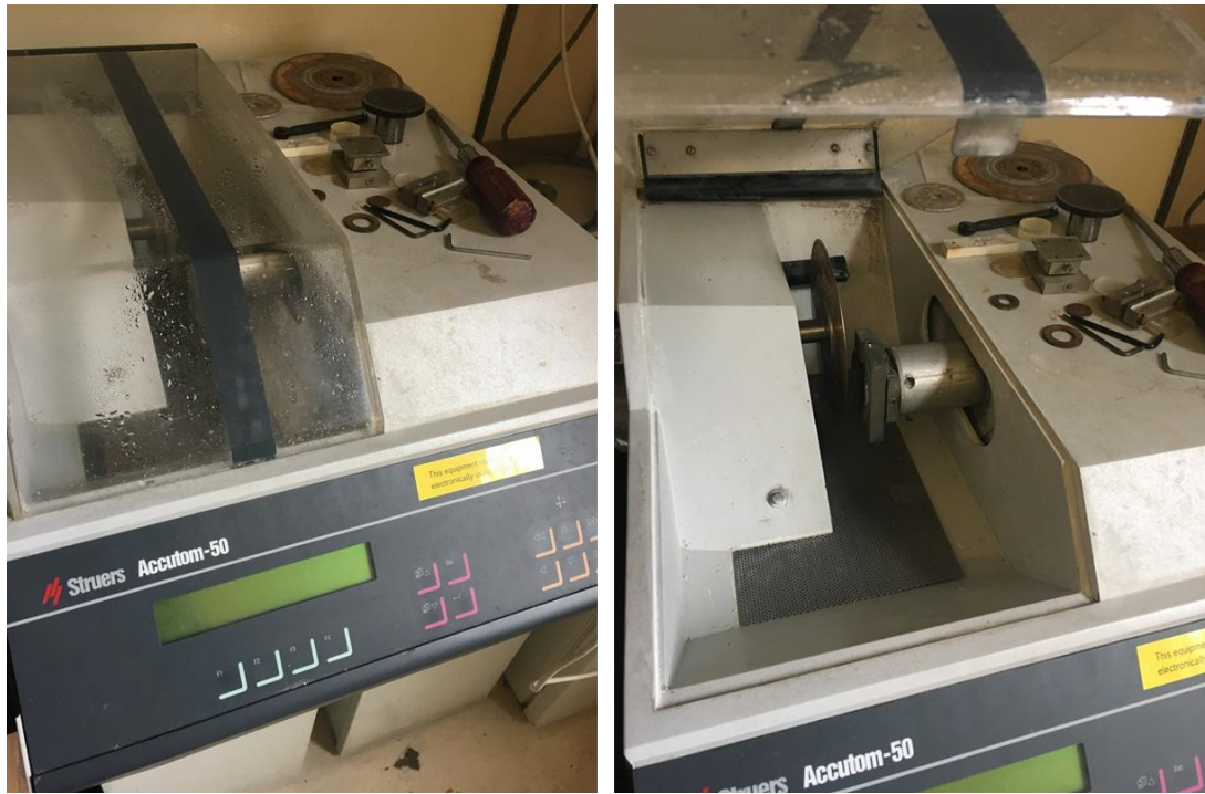
Figure 17. Accutom-50 saw used with diamond blade to cut glass.
