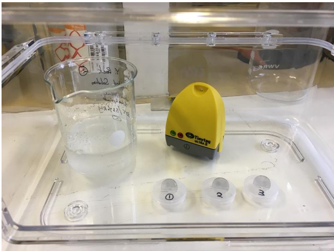
Figure 40. Air tight humidity chamber with saturated solution providing constant humidity and Tinytag device to record temperature and humidity.
