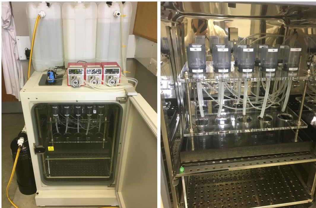
Figure 21. NuAire environment chamber set at 30 °C for static and dynamic immersion tests.
