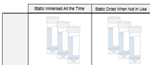
Figure 18. Figure of sample vials containing 20 mL of TW or dH 2 O to pictorially show how they were stored during static immersion test.
