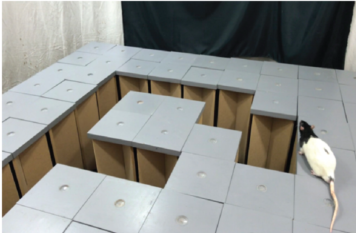
Figure S1: The maze environment used for the rat experiment, related to Figure 1. The environment consists of 100 removable maze modules with a black curtain over one of the surrounding edges to provide a single extra-maze cue. Reward can be dispensed at the goal module by filling the well with chocolate milk via polymeric tubing beneath the maze.
