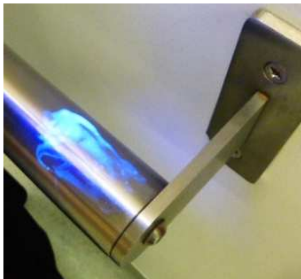
Figure 1.2 UV marker gel on a railing within a clinical space showing failure post-cleaning from a paediatric CICU.
