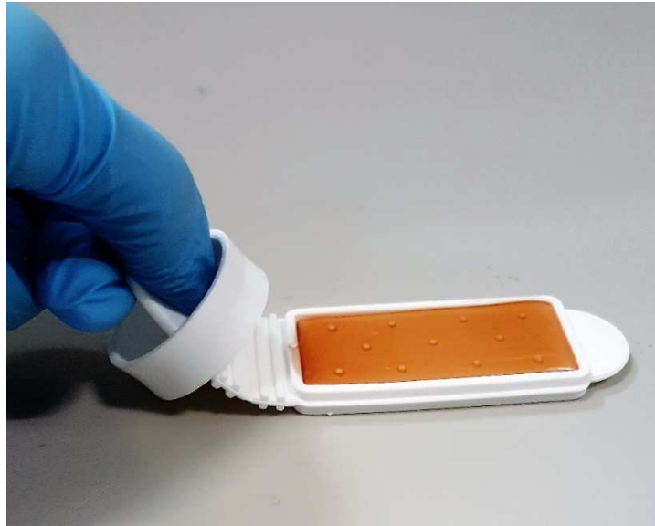
Figure 2.3 Use of a dipslide with selective agar to take a surface sample.
