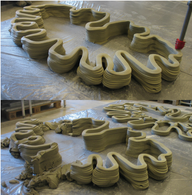
12 3D Concrete printing process and printing failure
