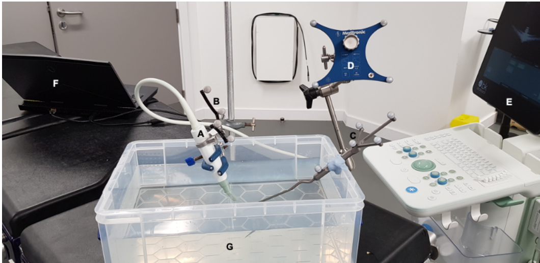
Figure 6.6: Ultrasound image calibration method. A: Ultrasound transducer (attached to a clamp for illustration purposes only). B: Medtronic SureTrack TM optical tracking marker. C: Medtronic Stylus. D: Medtronic reference frame. E: BK5000 Ultrasound machine. F: computer. G: water tank.
