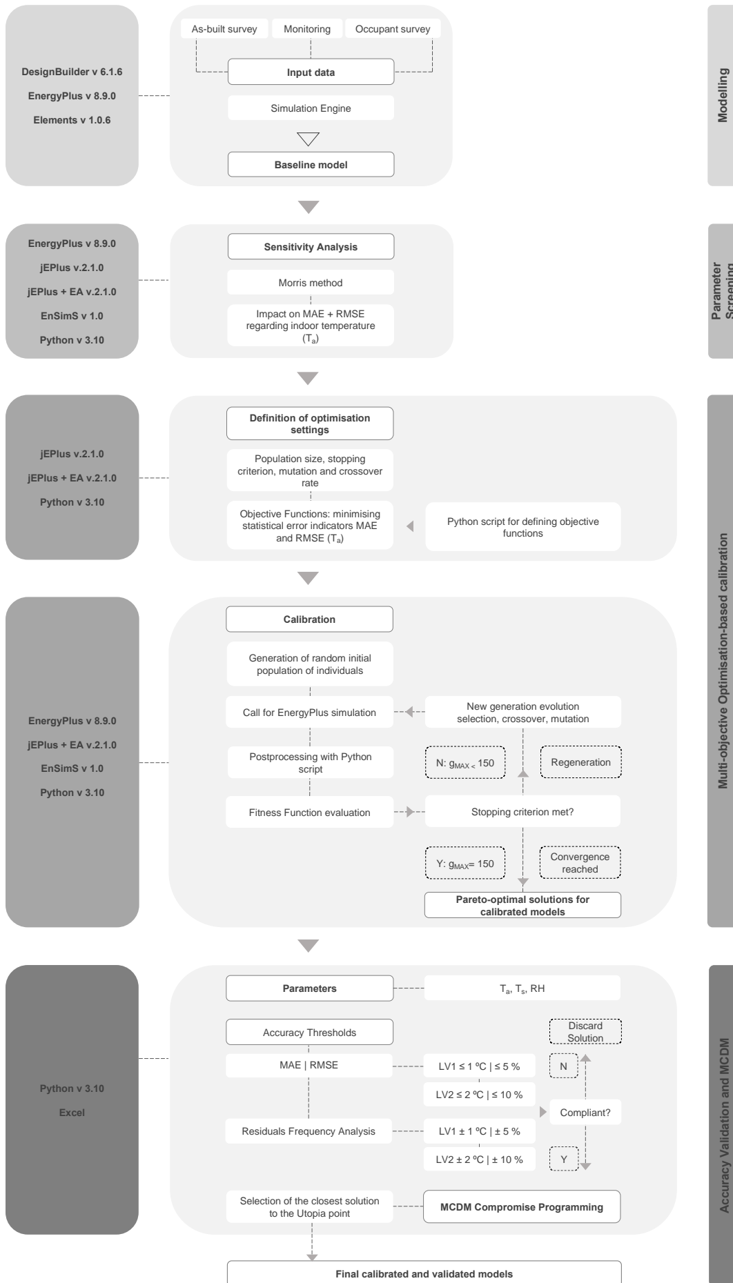
Fig. 3. Technical process for the calibration and validation of the vernacular case study models.
