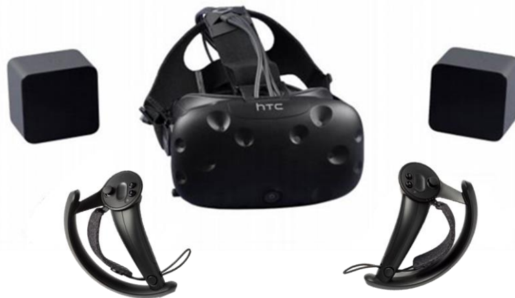
Figure 4.4. Composite image showing the HTC Vive headset with SteamVR tracking base stations (HTC Corporation, 2016) and Valve Index controllers (Valve Corporation, 2019).
