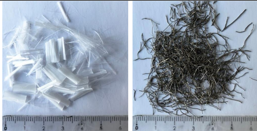
Figure 6-1 Images of (a) polyvinyl alcohol (PVA) and (b) recycled tyre steel (RTS) fibres.
