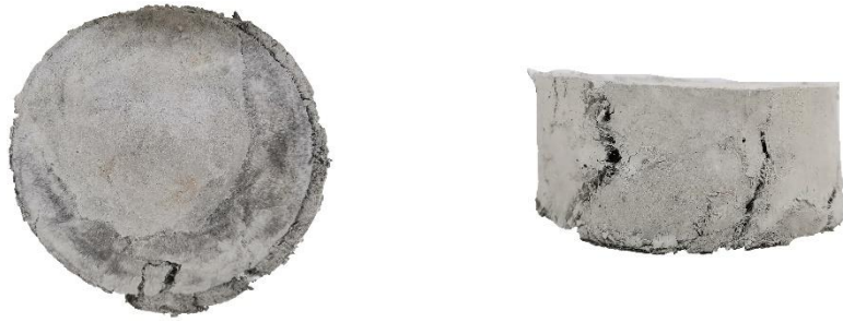
Figure 5-10 Typical failure patterns of SHGC cylinders
