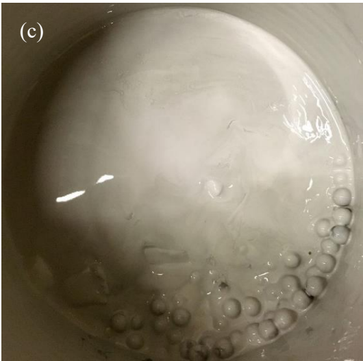
Figure 10. Angular grains after 20000 revolutions: a) tested in dry condition (RUN 2); (b) saturated with water (RUN 3); (c) saturated with clay-slurry (RUN 4); (d) saturated with silt-slurry (RUN 5) (each gravel grain has a diameter 20-30 mm)
