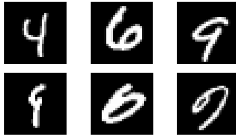
Figure 5.11: Representation of the test set digits for three classes (4, 6 and 9) in which the ensemble predictor is most certain/uncertain. The top row shows the digits with minimum uncertainty (all 100 members of the ensemble agree in the prediction). The bottom row shows the digits with highest uncertainty.
