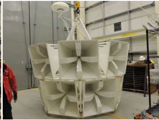
(b) The top ring antennas are mounted.
