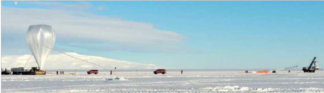
Figure 5.26: ANITA launch preparation setup. The Long Duration Balloon is inflated with helium (left), and a small test balloon (top left) is launched to monitor wind speed. The base of the Long Duration Balloon is attached to the spool vehicle; this balloon is connected to the ANITA payload (with a parachute interconnect), which is on the Boss (right).
