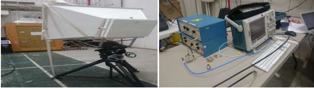
(a) Antenna positions for pulsing. The receiving antenna (closest) was adjusted in elevation and azimuth by the adjustable mount. The pulsing antenna (furthest) was mounted on an antenna crate. (b) The pulsing setup used an impulse generator unit as well as an oscilloscope to read out the data.
