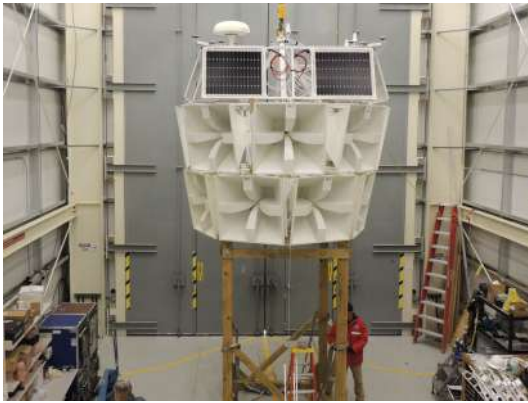
(c) A crane hook is used to lift the top ring of the payload so that the rest of the gondola can be constructed. The solar panels are fitted on top.
