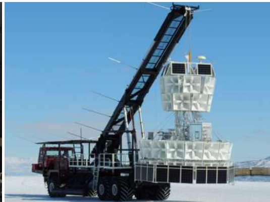
(f) The instrument box and SIP are fitted onto the payload deck. ANITA is then loaded onto the launch vehicle: the Boss .
