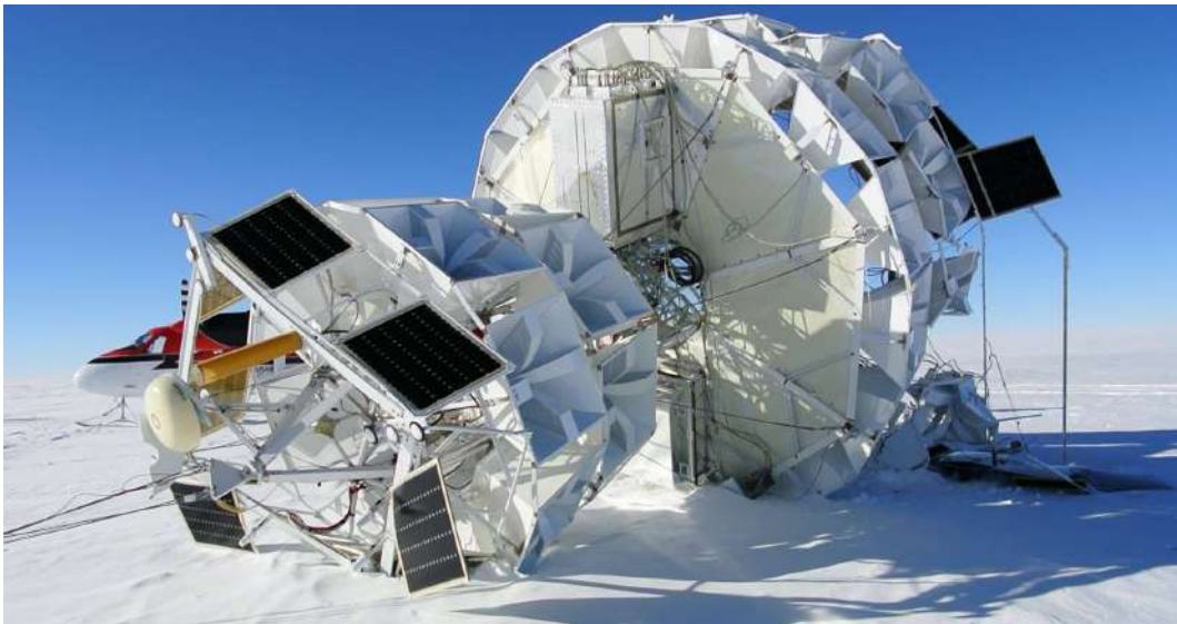
Figure 5.30: The ANITA-4 crash site. A team was dispatched to recover the hard drives and other components, such as the AMPAs. Photograph by Christian Miki.
