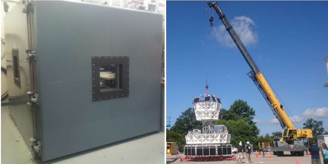
(a) The vacuum test: ANITA is subjected to vacuum conditions within the thermal-vacuum chamber. (b) The hang test: ANITA is suspended by a crane hook and checked to see if its core systems do not interfere with those of CSBF.
