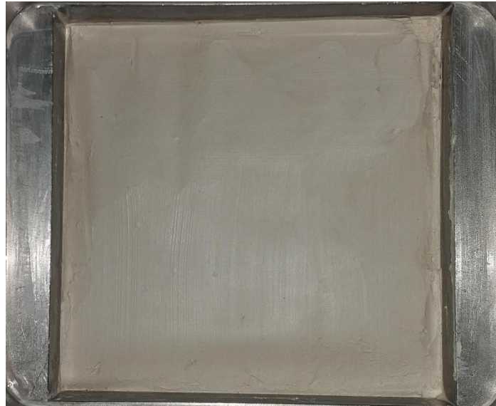
Fig.6a. Pure kaolin sample prepared in the shear box
