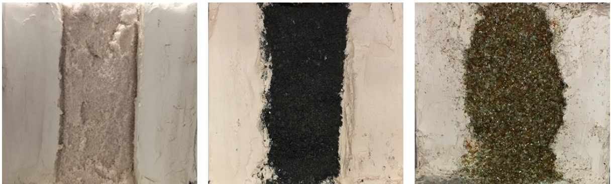
Fig.11. Post-shearing cross-section of the geocomposites under 25 kPa normal stress (NS-kaolin, MS-kaolin and CWG-kaolin geocomposite from left to right)
