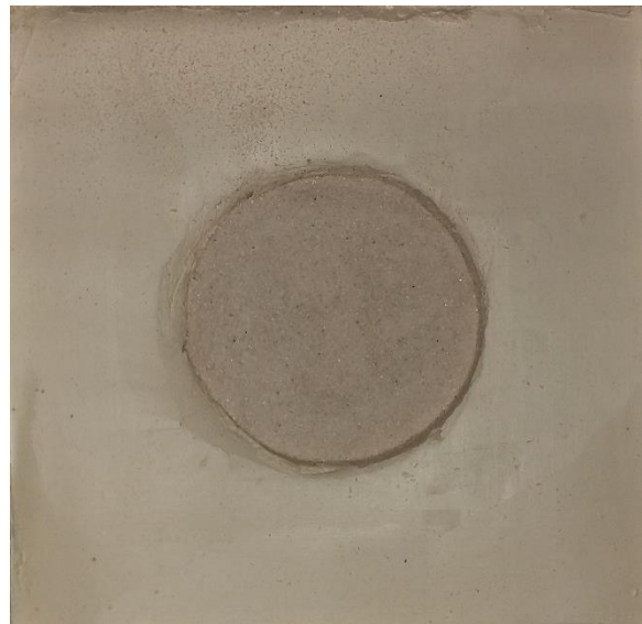
Fig.6b. NS-kaolin geocomposite prepared in the shear box
