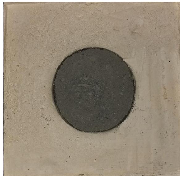
Fig.6c. MS-kaolin geocomposite prepared in the shear box
