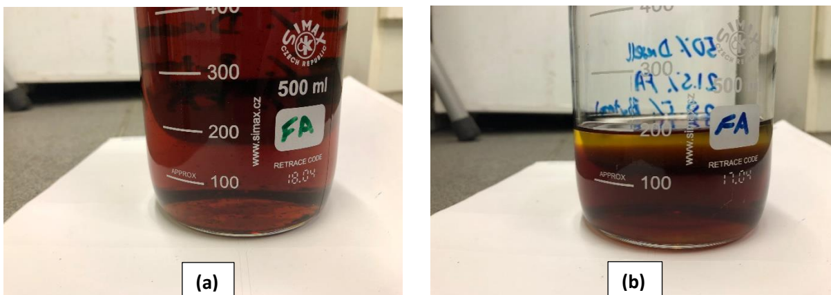
Figure 2.3: Comparison of 50:50 furfuryl alcohol blend with diesel having formed a homogenous mixture (a) and a visibly separated mixture (b)
