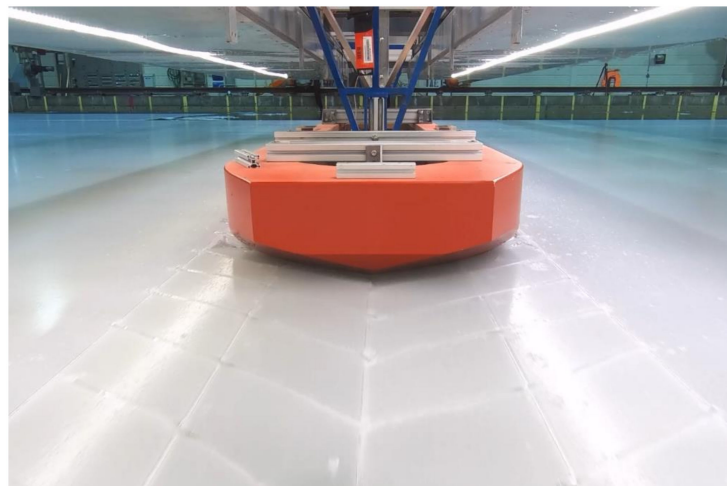
Figure 8. A model ship towed through presawn ice at the Aalto ice tank (photo taken by the first author).
