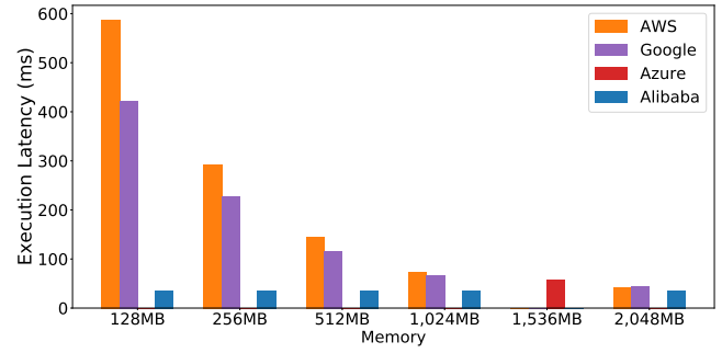
FIGURE 8 The execution latency for the memory-bound workload.
