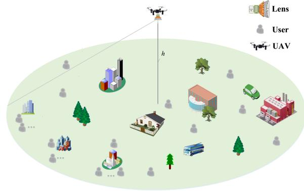
Fig. 2. Illustration of a UAV-enabled hybrid beamspace beamforming for multiuser mmWave communication systems.
