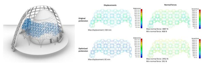
Figure 1. The distance to the target net under live loads is minimized by optimizing the tension in the outer cables.
