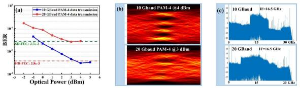
Fig. 2. (a) The BER performance for the 10- and 20 GBaud PAM-4 signals after wireless transmission. (b) Eye diagrams of 10 GBaud PAM-4 signal at 4 dBm optical power and 20 GBaud at 3 dBm. (c) The electrical spectra of the 10- and 20 GBaud PAM-4 signals after the down conversion.
