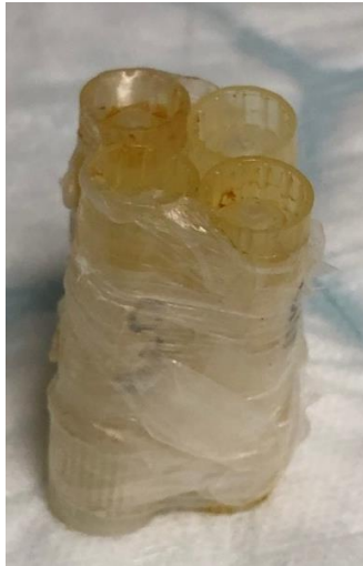
Figure 3.1 Phantom containing air, water, ethanol, and wax
