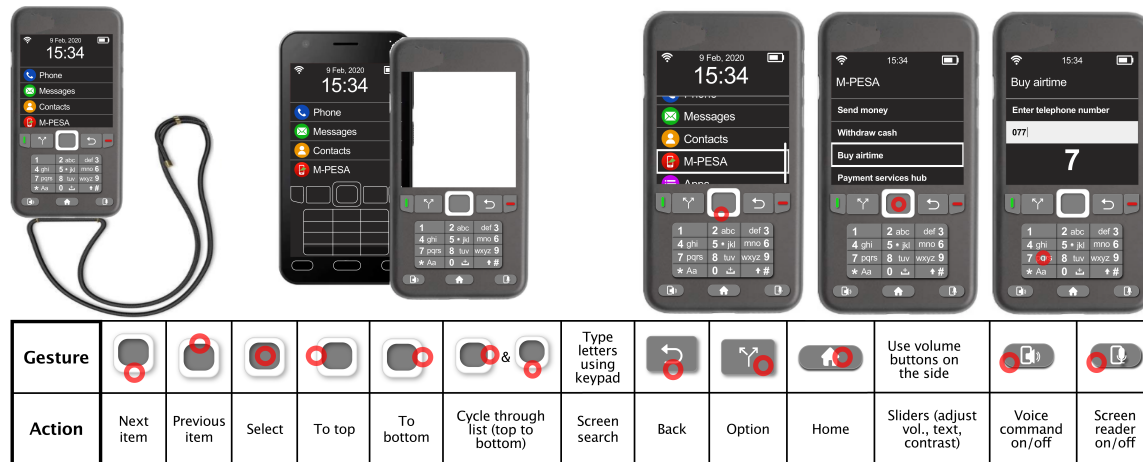
Fig. 1. Design and interactions of the CaseGuide concept
