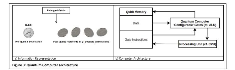
Designing a Quantum computer, guided by our computation mechanisms (section 2): a) *Information* - Qubits represent computation; b) *Structure/processing* – uses Quantum entanglement to build structure and Quantum processor interprets the computation; c) *Control* – a Quantum control mechanism might use *explicit* memory addresses; and d) *Communication* – a Qubit memory supports *multicast*.
