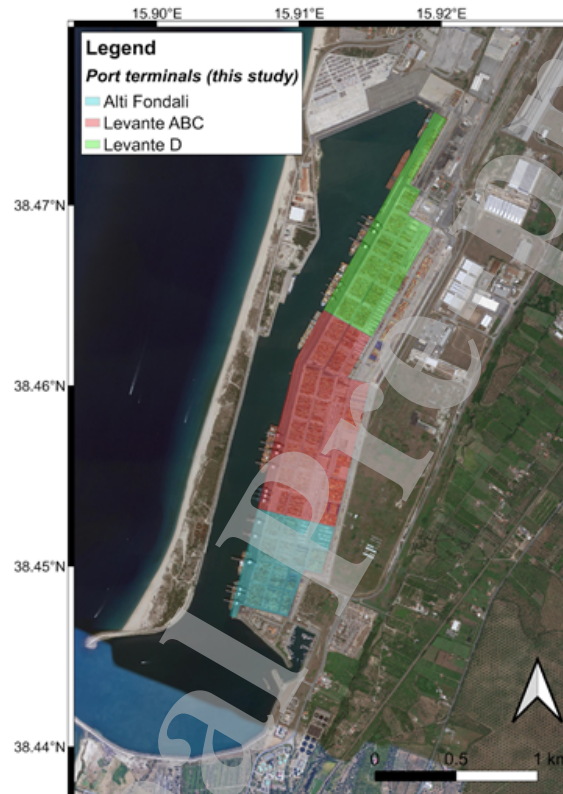
Figure 2: Map of the case-study Gioia Tauro port, which is a complex system of various components including wharves, cranes, an electric power system, strategic buildings, etc. The three main terminals considered in this study, namely Alti Fondali, Levante ABC and Levante D, are highlighted in the map.
