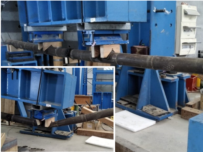
Fig. 4. Typical test setup and failure mode (inset) for short loading saddles
