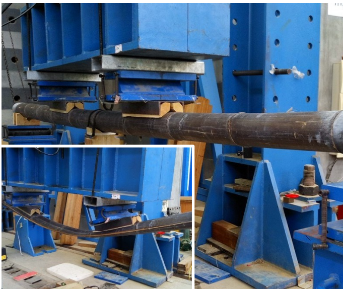
Fig. 5. Typical test setup and failure mode (inset) for long loading saddles
