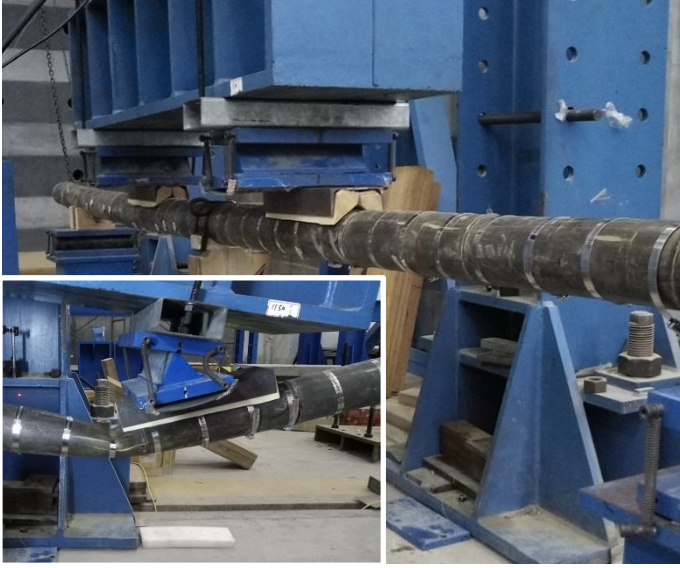
Fig. 6. Typical test setup and failure mode (inset) for long loading saddles with reinforcement
