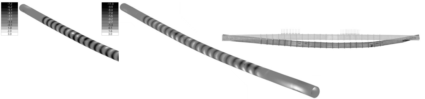
389 Fig. 16. \sigma_{ti\perp} (left), \sigma_{to\perp} (right) for reinforced pole ML3 with long loading saddles
