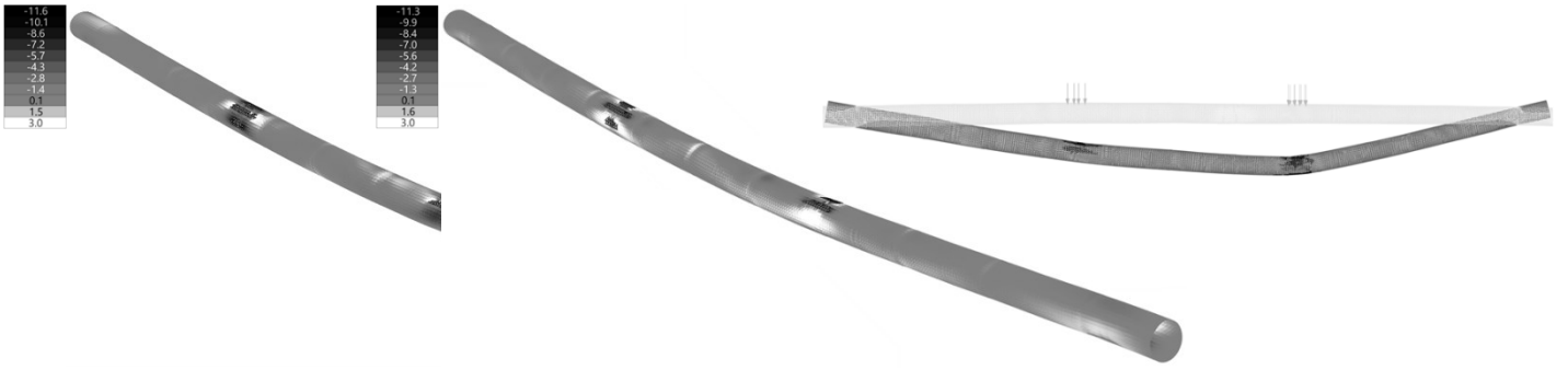
375 Fig. 15. \sigma_{ti\perp} (left), \sigma_{to\perp} (centre) and failure mode (right) for pole ML3 with short loading saddles
