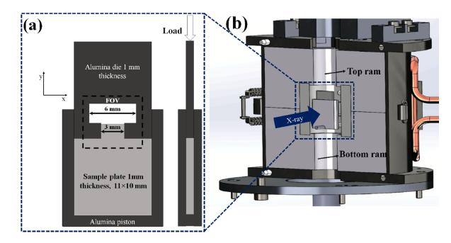
112 Fig.1. Experimental setup used in I13-2 beamline: (a) Cross-sectional view and side view of the assembly showing
