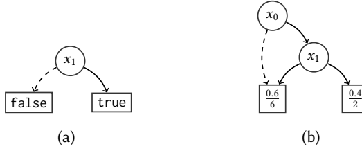
Fig. 12. (a) shows an example representation of an assertion that depends on a 3-bit integer symbolic. (b) shows the MTBDD representation of its distributions.
