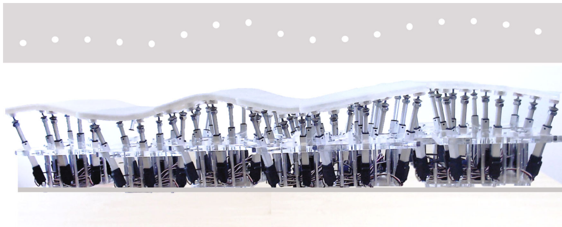
Fig. 4 Movable shape display. Trace of the prototype mounted on a mobile platform that allows a person to feel a shape as it moves across space.
