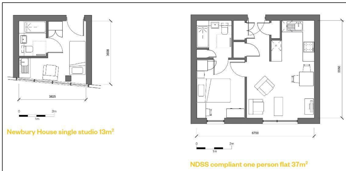
Figure 1: Comparison between the smallest one-person studio in Newbury House and a one bed flat that complies with the NDSS (Source: Levitt Bernstein, 2019)
