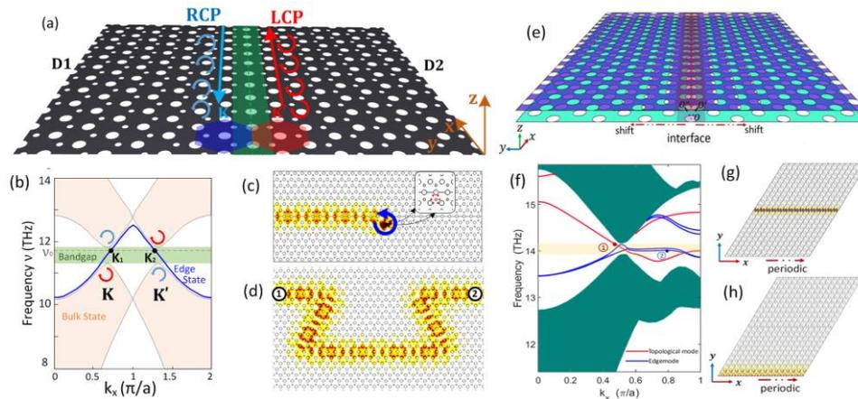
**Figure 1.** Two types of graphene crystal waveguides possessing plasmonic topological valley-Hall interface modes. (a)-(d) Band diagram and topological propagation features of a single-layer graphene plasmonic crystal waveguide. (e)-(d) Same as in (a)-(d), but for a bi-layer graphene plasmonic crystal waveguide.
