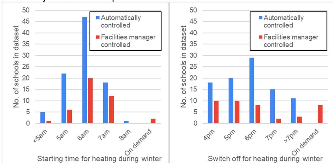
**Figure 7 - Winter heating on and off times**
