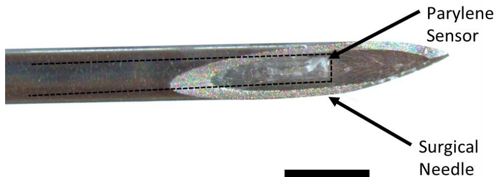
Figure 3.27 – Microscope image of an assembled parylene pressure sensor inserted through the inner lumen of a surgical needle. Dashed line indicates the position of the sensor. Scalebar is 1 mm.
