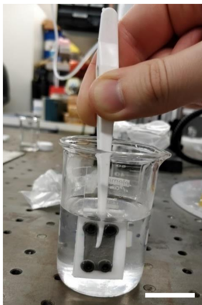
Figure 3.13 - Photograph of the capillary functionalisation jig being placed in a beaker of IPA with complimentary PTFE tweezers. Scalebar is 2 cm.
