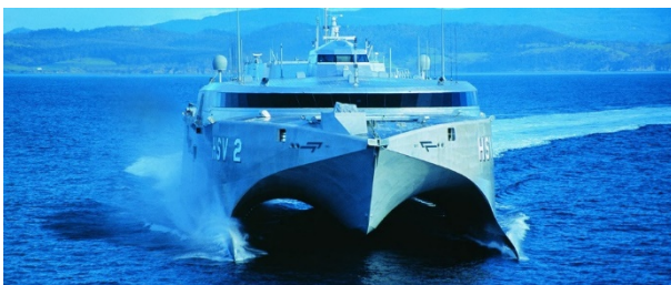
Figure 1: HSV-2 SWIFT, a 98-meter wave piercing catamaran built in 2003 (Hull 061) (Incat.com.au, 2019).
