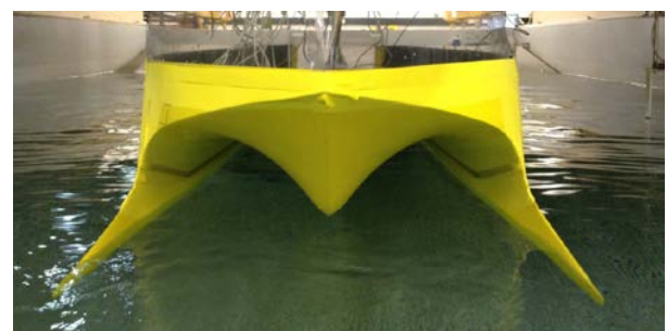
Figure 3: The centre bow of a model wave piercing catamaran (Shabani et al. , 2017).
