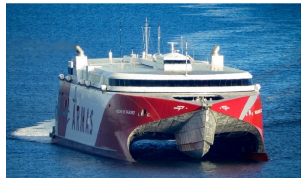
Figure 2: Volcan De Tagoro, A 111- m wave piercing catamaran built in 2019 (Hull 091) (Incat.com.au, 2019).
